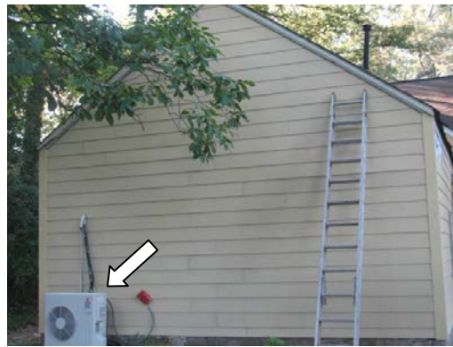
Figure 12. Photograph of the rear view of the addition. The mini-split outdoor unit is highlighted in the image by the arrow.
