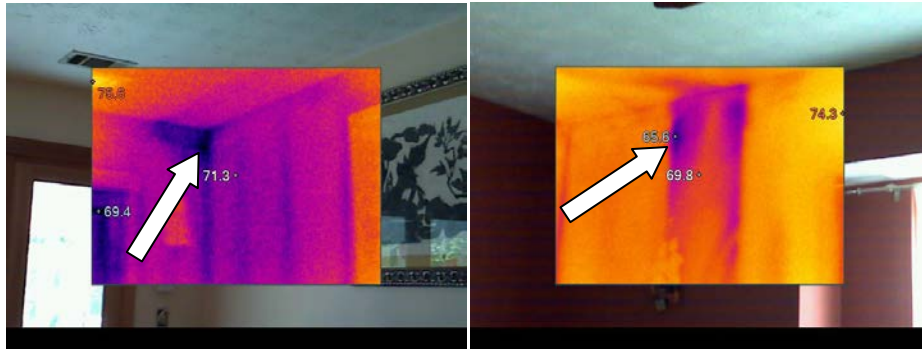
Figure 55. Thermal image highlighting insulation voids in exterior walls.
