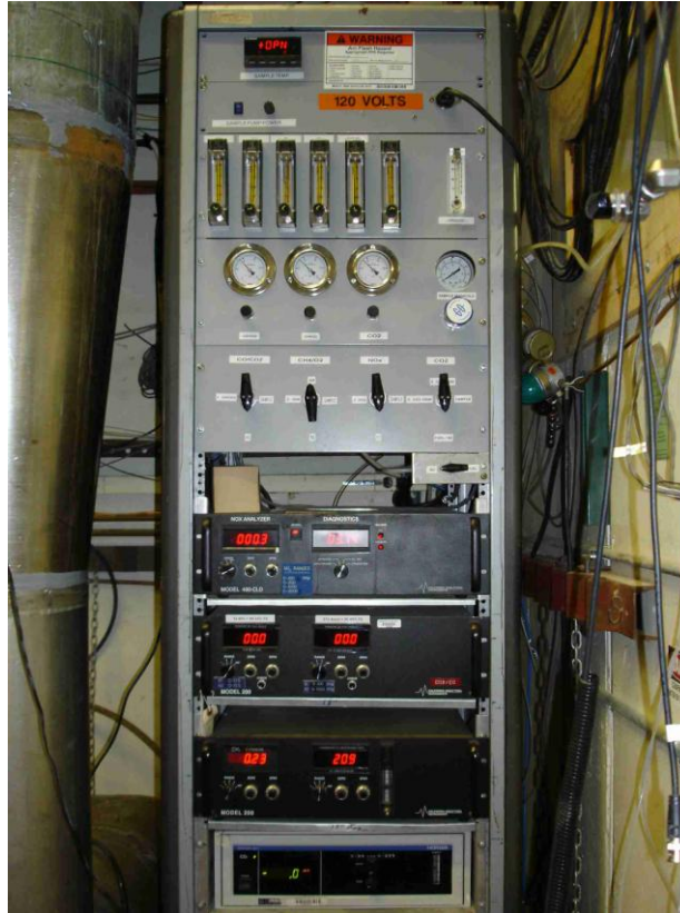
Figure 15: Test cell emissions sampling system.
