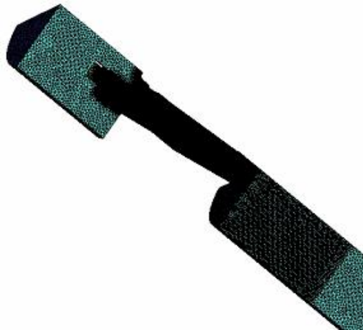
Figure 16: LES Mesh of the 1/5th sector CFD simulation with enforced rotational periodicity.
