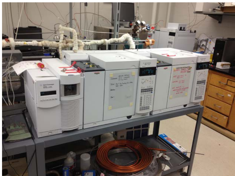
Analytical 2 (Agilent 7890A GC with 5975C MSD) and Analytical 3 (Agilent 7890A GC)
