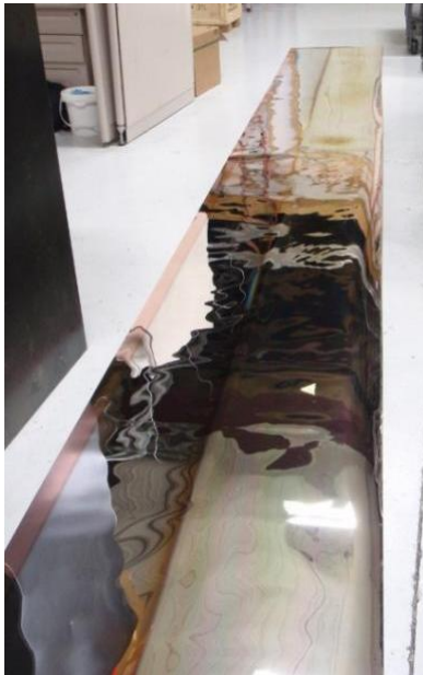
Figure 7. Reflective film. Left side is bare silver film and right side is Alumina coated film
