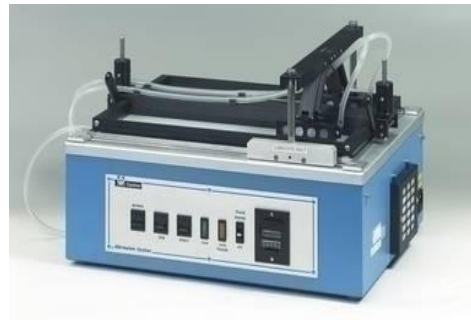
Figure 22. ASTM D2486 Two-Channel Wet Abrasion Scrub Tester
