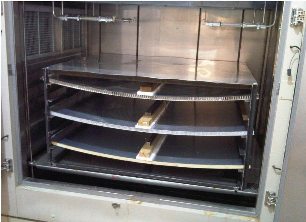
Figure 14. Panels in Elevated Temperature Chamber
