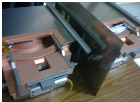
Figure 9. E-beam magnetic field test with a piece of \mu -metal placed in between the sources
