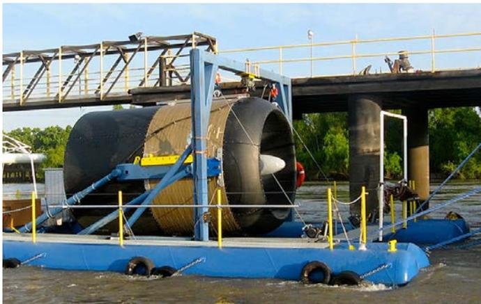
Hydrokinetic turbine generator deployed on floating mount in Mississippi River. *Photo from Free Flow Power Corporation.*
