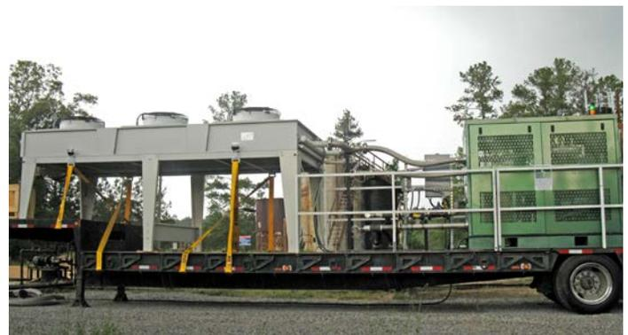
The ElectraTherm Green Machine generates electricity from the waste water discharged by oil and gas production. *Photo from ElectraTherm, Inc.*
