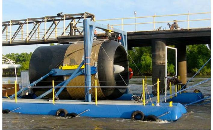
Hydrokinetic turbine generator deployed on a floating mount in the Mississippi River. *Photo from Free Flow Power Corp*
