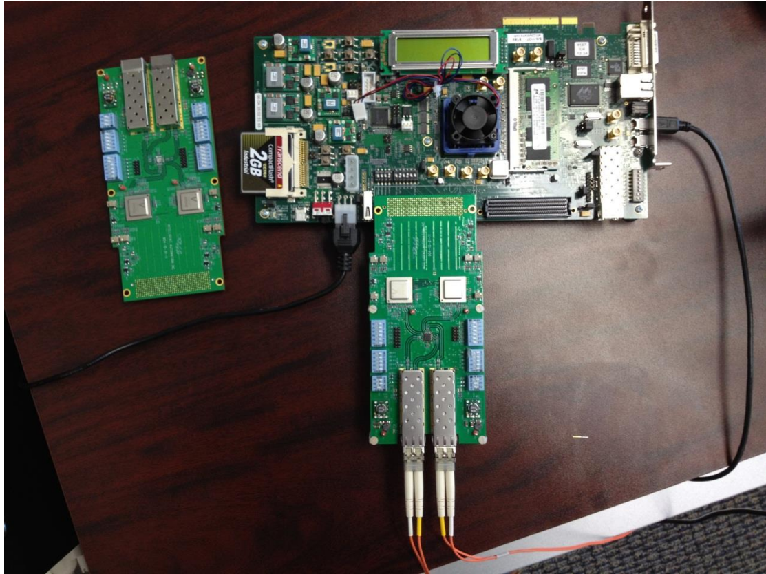
Figure 7 10 Gig Capture PHY and Main board
