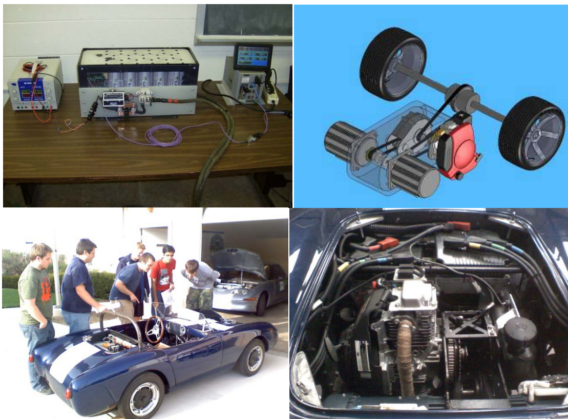
Figure 8: Top Left – Lithium battery pack, top right – drive train schematic, lower left – HIL class during lab 5, lower right – photo of drive train installed
