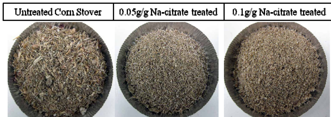
Figure 6. Comparison of 0.05g/g and 0.1g/g Na-citrate treated samples to the untreated corn stover.
