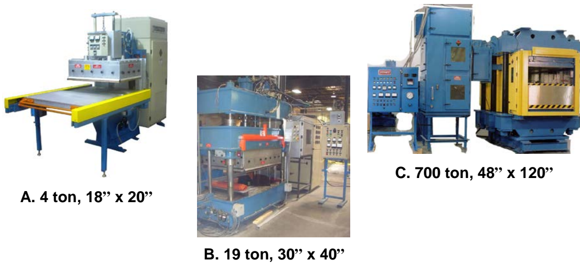
Figure 11. Photographs of RF presses suitable for RF Lamination. A) lab-scale press used in Phases I & II work. B) pilot press used in Phases II & III work, C) large press sold by Thermex Thermatron for another application, demonstrating the existing scalability of the RF press technology.
