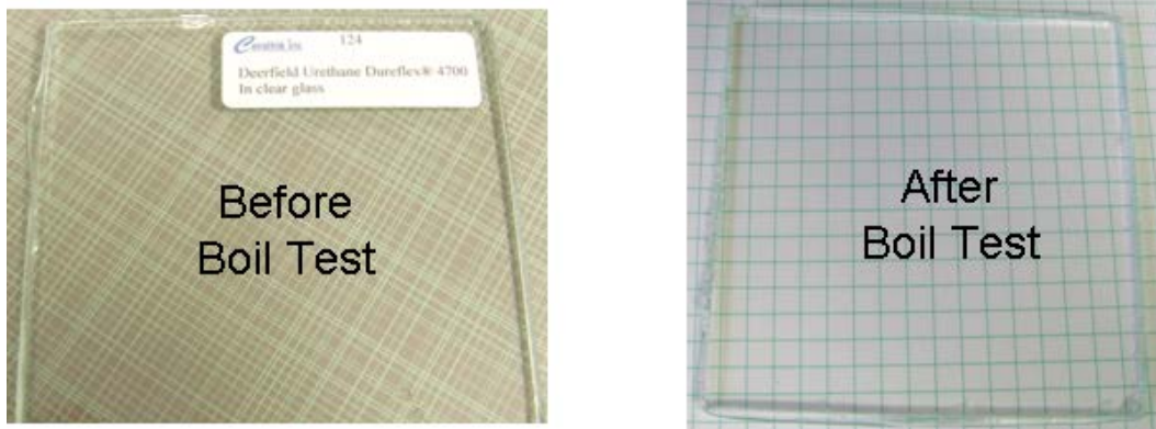
Figure 3. Before and after photographs of 1.5 year room-temperature aged thermoplastic polyurethane (TPU) RF-laminated sample, subjected to boil test – 2 hours in boiling water. The sample passed the test, retaining defect free clarity after boiling, with no development of bubbles, delamination, or haze.
