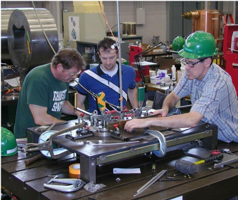
Fig. 7. Coil winding.
