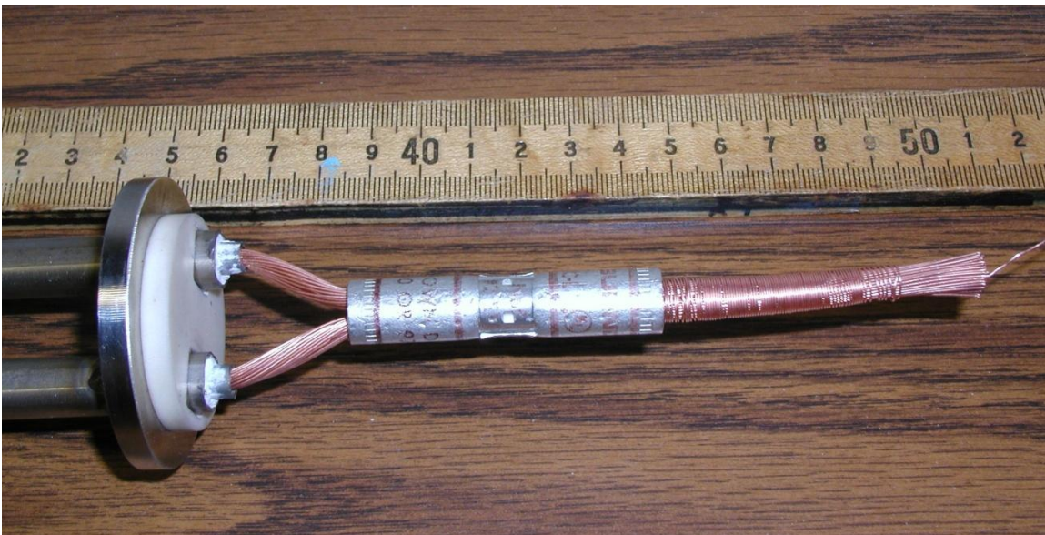
Fig. 11. Test splice.
