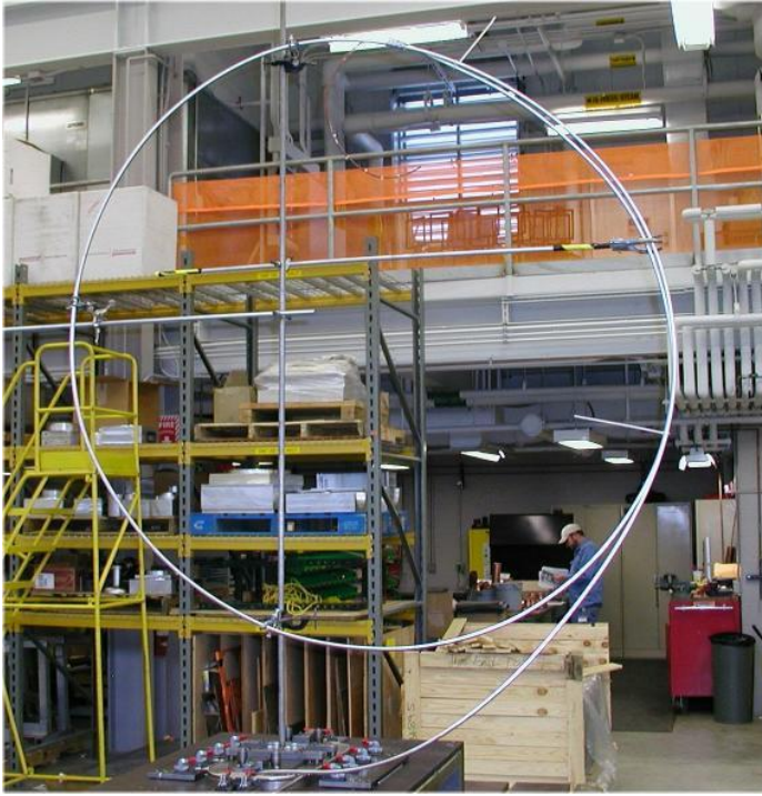
Fig. 6. The conductor for the second layer is supported above the winding fixture.
