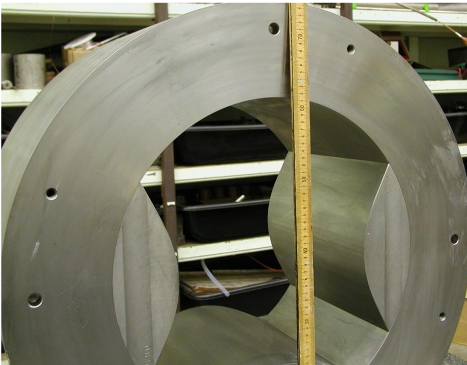
Fig. 4. Magnet iron with one pole tip removed.
