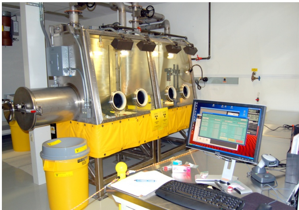
Figure 6. The CCL glove box used to visually inspect irradiated graphite samples, perform dimensional measurement, and repackage samples for storage in the irradiated graphite vault located in Lab C-19.
