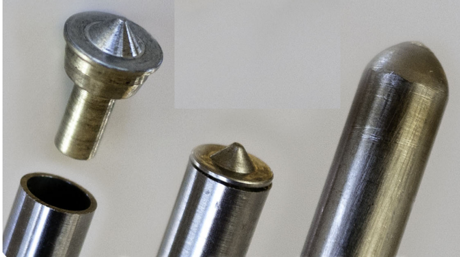
Figure 1. Progression from fuel element pieces to finished weld
