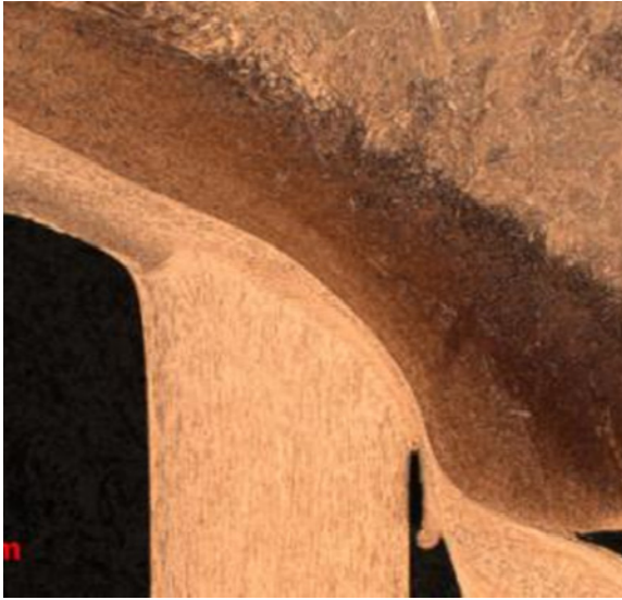
Figure 4. Bond line between end plug and tube
