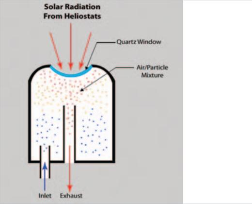
This conceptual schematic shows a small particle solar receiver. Concentrated radiation from the heliostat field is absorbed directly in a gas-particle suspension rather than on the receiver walls. The carbon nanoparticles oxidize as they transit the receiver, resulting in a clear gas stream exiting toward the turbine. *Illustration from San Diego State University*
