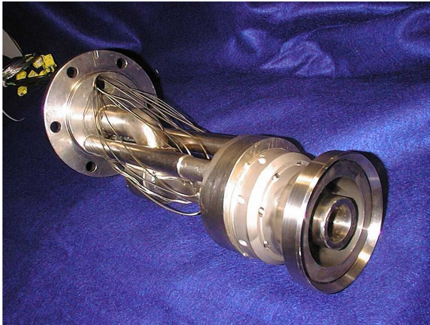
Figure 8: Photograph of modified T70 premixed fuel/air injector hardware, with RCL ® Pilot
