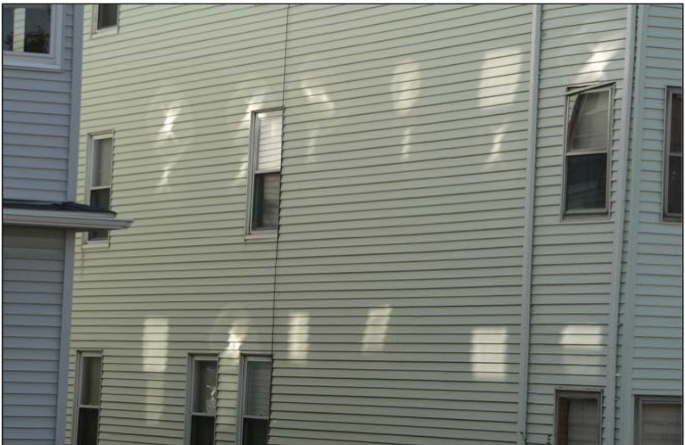
Figure 13. Image of varying IGU reflection shapes from a series of double-hung windows on a house that is ~30 ft. away and parallel to the reflecting glass surfaces
