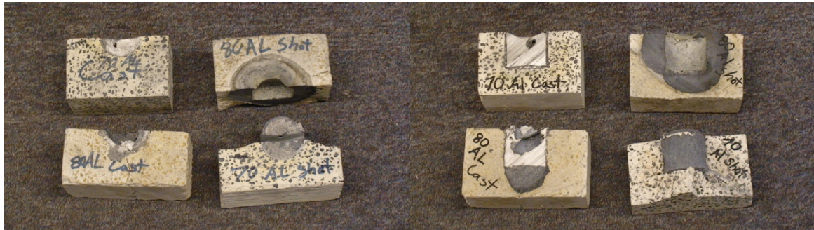
Figure 44. MINTEQ Refractory Samples Following Alcoa Standardized Cup Testing at MS&T
