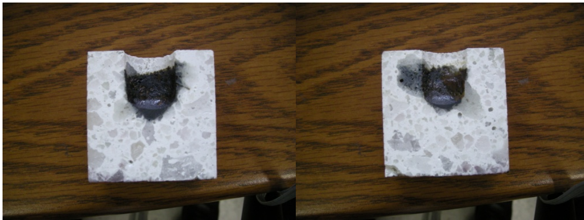
Figure 57. Coal Smelt Cup Test Samples of MINTEQ Developed Refractories for Coal Gasification
