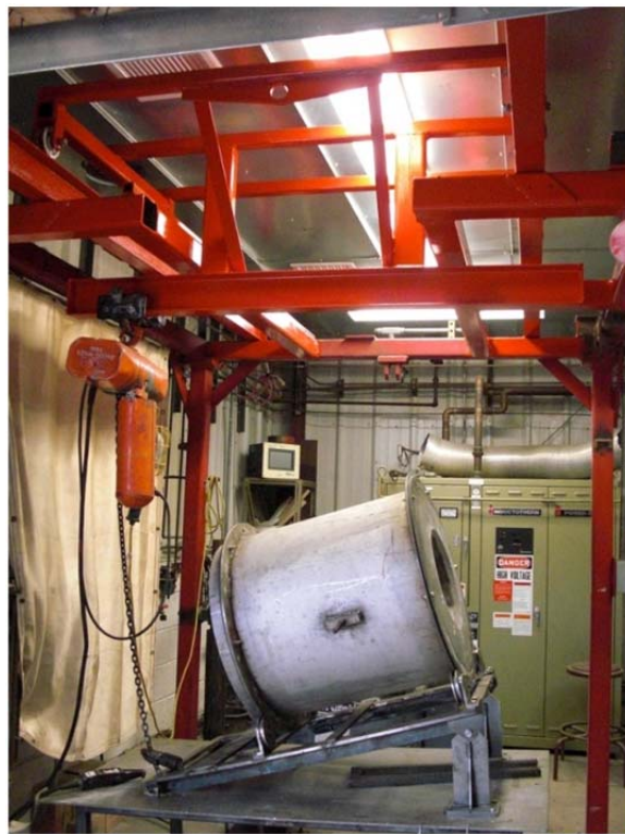
Figure 99. MINTEQ Rotary Furnace Simulation Test Schematic and Actual Picture of Completed System
