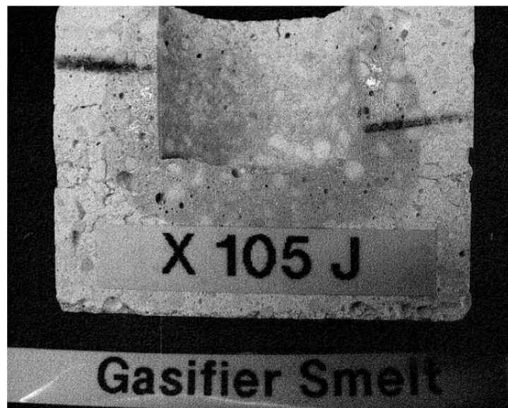
Figure 60. Smelt Testing of Experimental Refractory Spinel Former for Black Liquor Gasifier Application
