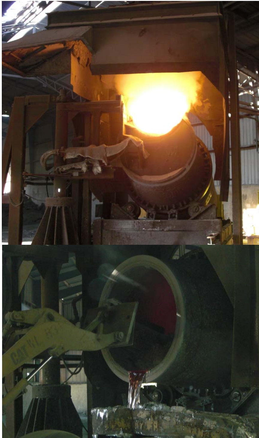
Figure 105. Aluminum Rotary Dross Furnace at Newco Metals (Bedford, IN) in Operation
