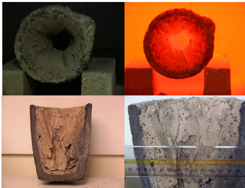
Figure 101. Spent Refractory Crucible Repair Material/Technique Adhesion Study Results for Aluminum Industry Applications
