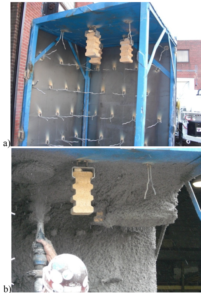
Figure 103. Pictures of Insulating Shotcrete Demonstration Showing Form Before Shooting (a) and Form During Shooting (b)
