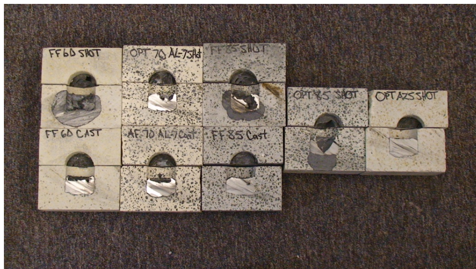
Figure 45. Materials After Steam Aluminum Cup Testing
