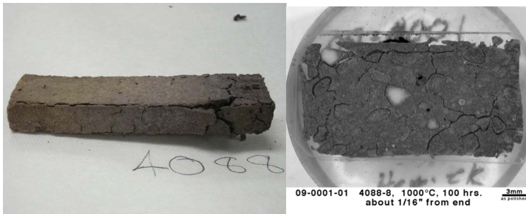
Figure 63. Examples of Black Liquor Smelt Immersion Testing Results for Industrial Samples
