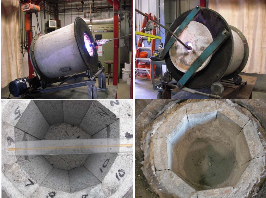
Figure 100. Rotary Furnace Simulation Test System During Testing and Pictures of Lining Before and After Aluminum Refractory Test
