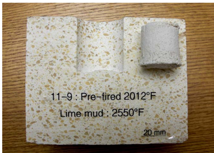
Figure 56. Lime Smelt Cup Exposure Tests Performed on Final Version of Spinel Forming Composition for Use in Lime Kilns
