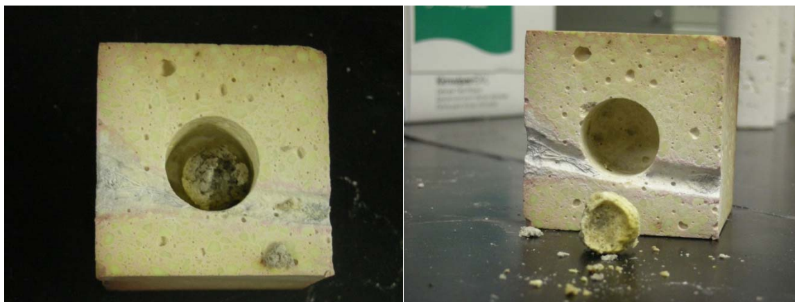
Figure 53. ORNL Lime Corrosion Cup Testing of Spinel Former (B) Material
