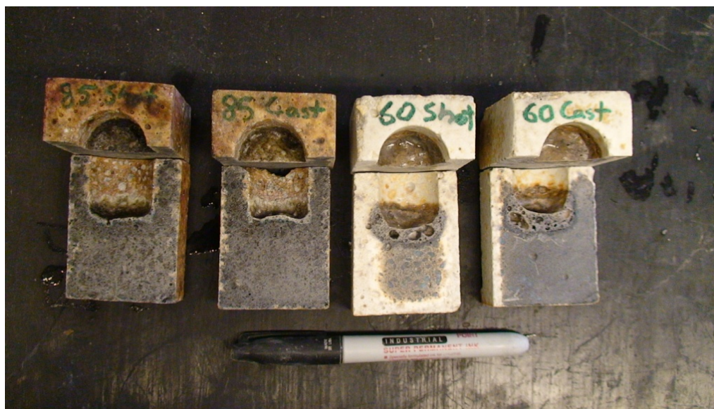
Figure 47. MS&T Lime Corrosion Cup Test Results
