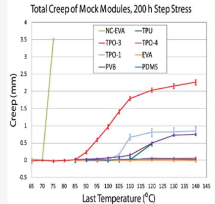
Test results of creep levels of various PV module types.
