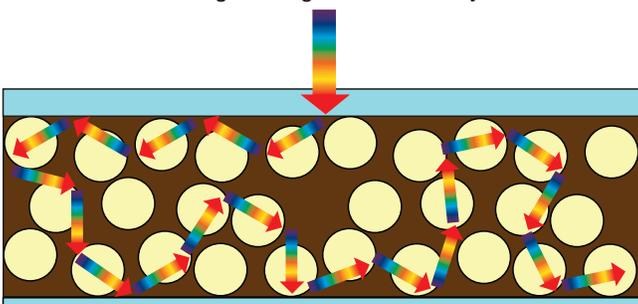
*Schematic of light scattering within the disordered inverse opal structure showing a nearly tenfold increase in the path length, or the distance traveled by light, through the film. Illustration by Nathan Neale, NREL*
