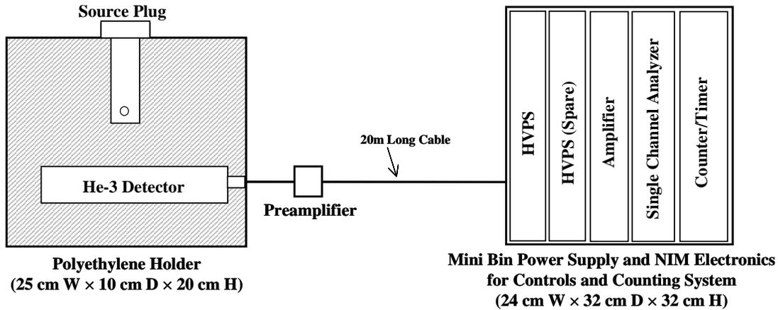
**Fig. 4. Main components of the NDS: Polyethylene plug holder, mini bin power supply and NIM electronics, preamplifier, and 20-m cable.** The plug holder contains a neutron detector, a high-efficiency  $^3\text{He}$  neutron counter wrapped with a cadmium sheet (manufactured by G.E. Reuter-Stokes, model RS-P4-0806-207).
