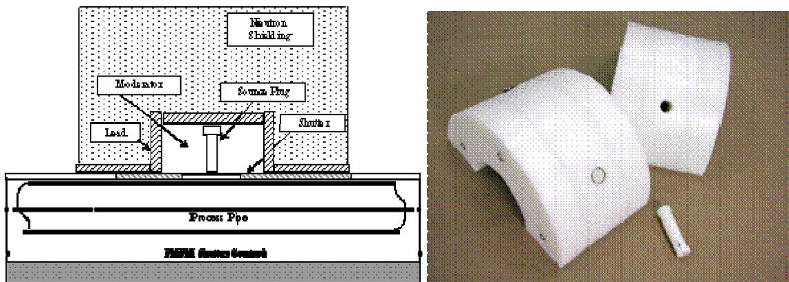
Fig. 3. Location of the FMFM sources inside the source modulator (left) and the polyethylene source plug housing the  $^{252}\text{Cf}$  neutron source (right) prior to installation in the source moderator [1].
