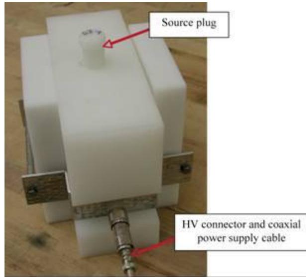
**Fig. 6. Detail view of the NDS source plug holder showing the FMFM source plug and the high-voltage connector used for the detector signal and to supply high voltage to the  $^3\text{He}$  counter located inside the plug holder.**
