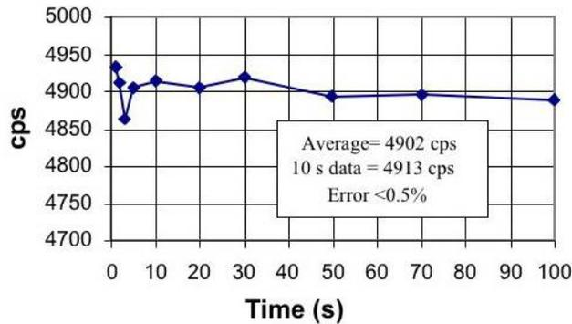
**Fig. 7.** NDS measurement count rate at various data collection times. A 10-s measurement time is sufficient to take the data. It yields about  $\leq 0.5\%$  uncertainty (error) from the average count.
