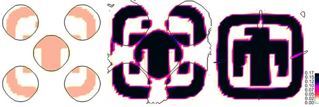
Figure 64 Results of closed-feature simulations under the patterned template shown in Fig. 5. The dark green curves represent the location of the liquid-air lubrication interface, while the color scheme represents the relative saturation, S\phi . In these figure (a) is at t = 10^{-6} s, (b) is at t = 12 s, and (c) is at t = 920 s.
