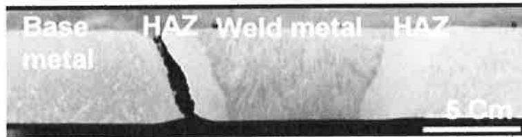
Figure 7. Type IV failure on the grain boundaries in the fine-grained HAZ in weld joint of modified 9Cr-1Mo steel.
