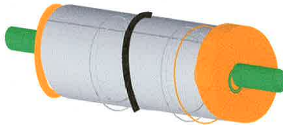
Figure 10. Schematic showing fixture design for circumferential butt welding.
