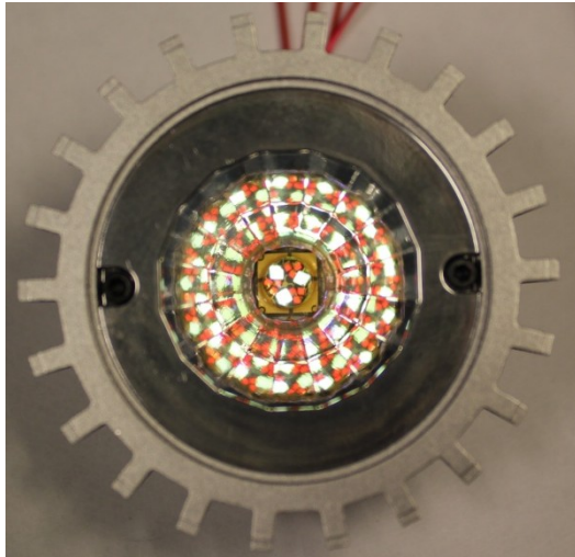
Figure 8. Photographs of the lamp with a metalized reflector optic. The diffuser cover is removed for clarity.
