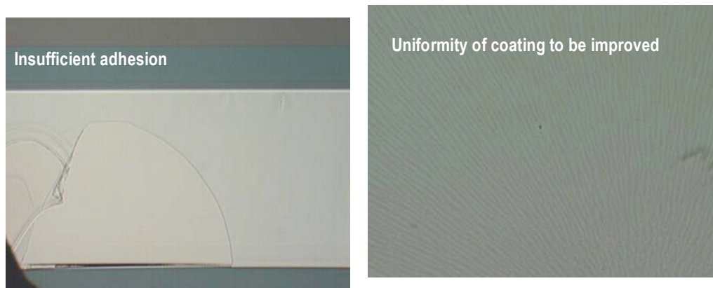
Figure 3. Pictures of PHMS-OH thin film coated on Al-Mg alloy surface before process optimization. Left: PHMS-OH film peeled off substrate due to insufficient adhesion. Right: non-uniform film.
