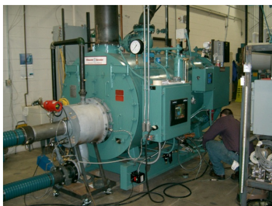
Figure 5. 80 HP Laboratory Super Boiler and Test Data
