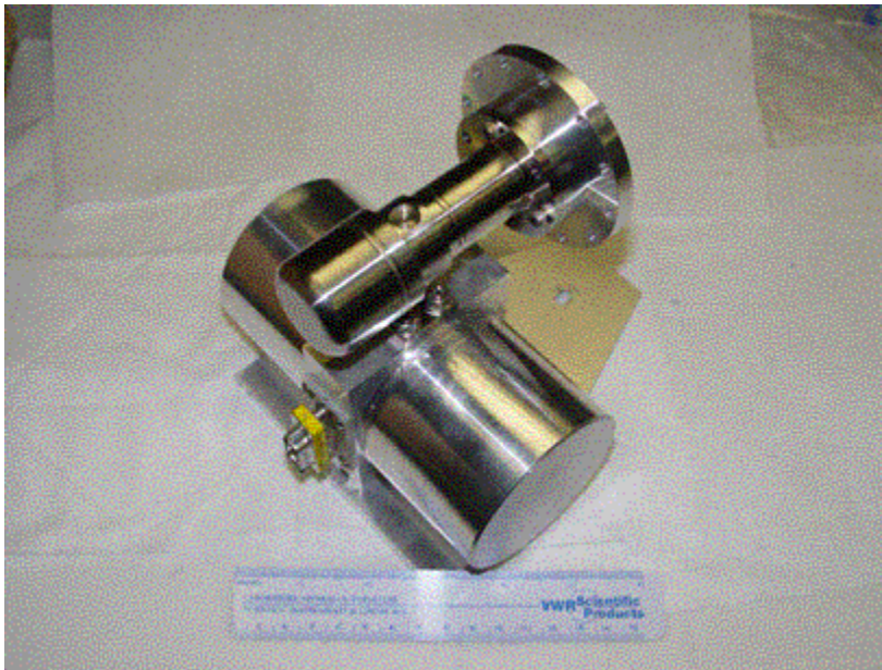
Figure 5. Hymatic tandem cryocooler.
