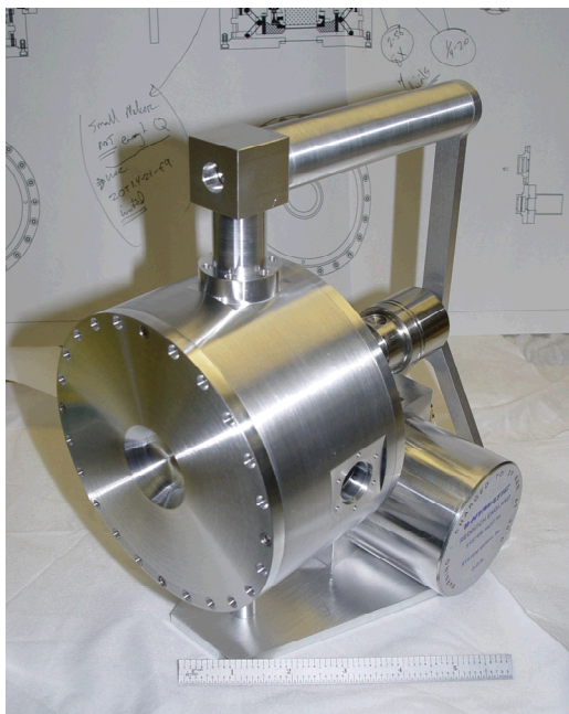
Figure 1. CryoFree: a mechanically-cooled, high-resolution, gamma-ray spectrometer.
