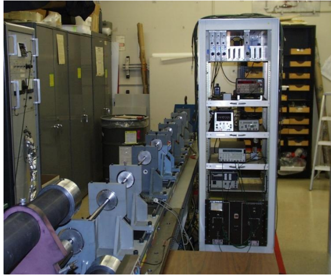
Figure 2. LLNL SHPB compression experiments.
