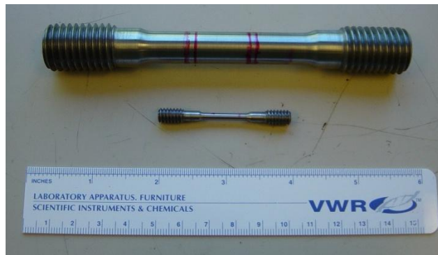
Figure 3. Smooth round NDI specimens- 0.5 in (1.27 cm) and 0.113 in (0.287 cm) diameter configurations.
