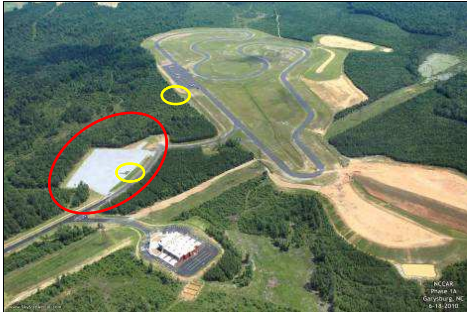
Figure 9: Paddock Area Awaiting Electrical Outlets (red) & Transformer Locations (yellow)
