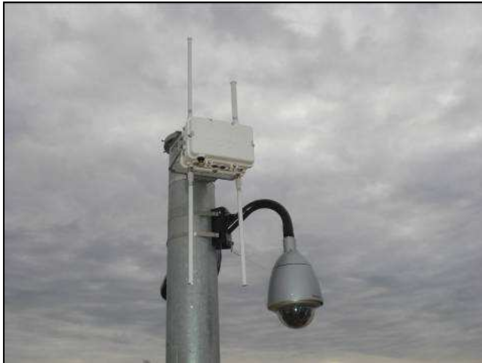
Figure 58: Access Point Detail (and PTZ Video Camera)
