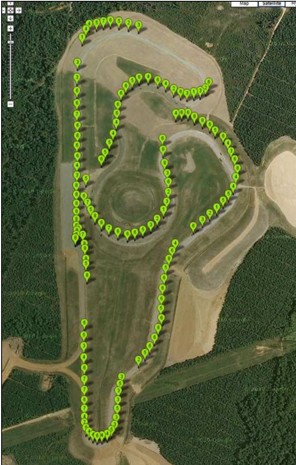
Figure 62: WiFi Coverage / Bandwidth Test using iperf (50mph counter clockwise)
