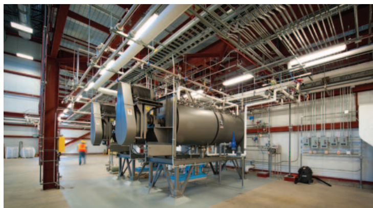
The IBRF's new enzymatic hydrolysis reactors can handle high solids – a key factor in reducing conversion costs.
