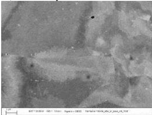
Figure 8. SEM micrographs of pristine and irradiated e-brite steel (Fe-26Cr-1Mo) using a 30MeV copper ion beam at room temperature. (experiment performed at SNL) Note the pronounced phase separation in these backscattered electron images.
