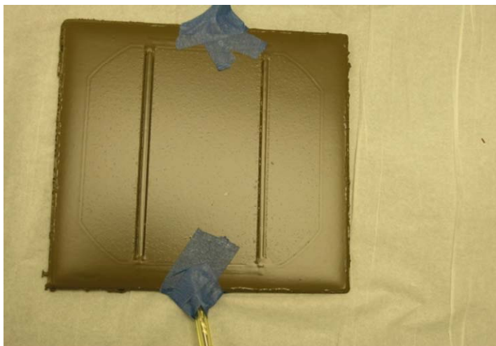
Figure 8. Photograph of backside of mini-module coated with refinish primer ARP and LT-1 top coat after 1000 exposure hours in damp heat test. Visual inspection reveals delamination and corrosion along the metal tabbing interface.
