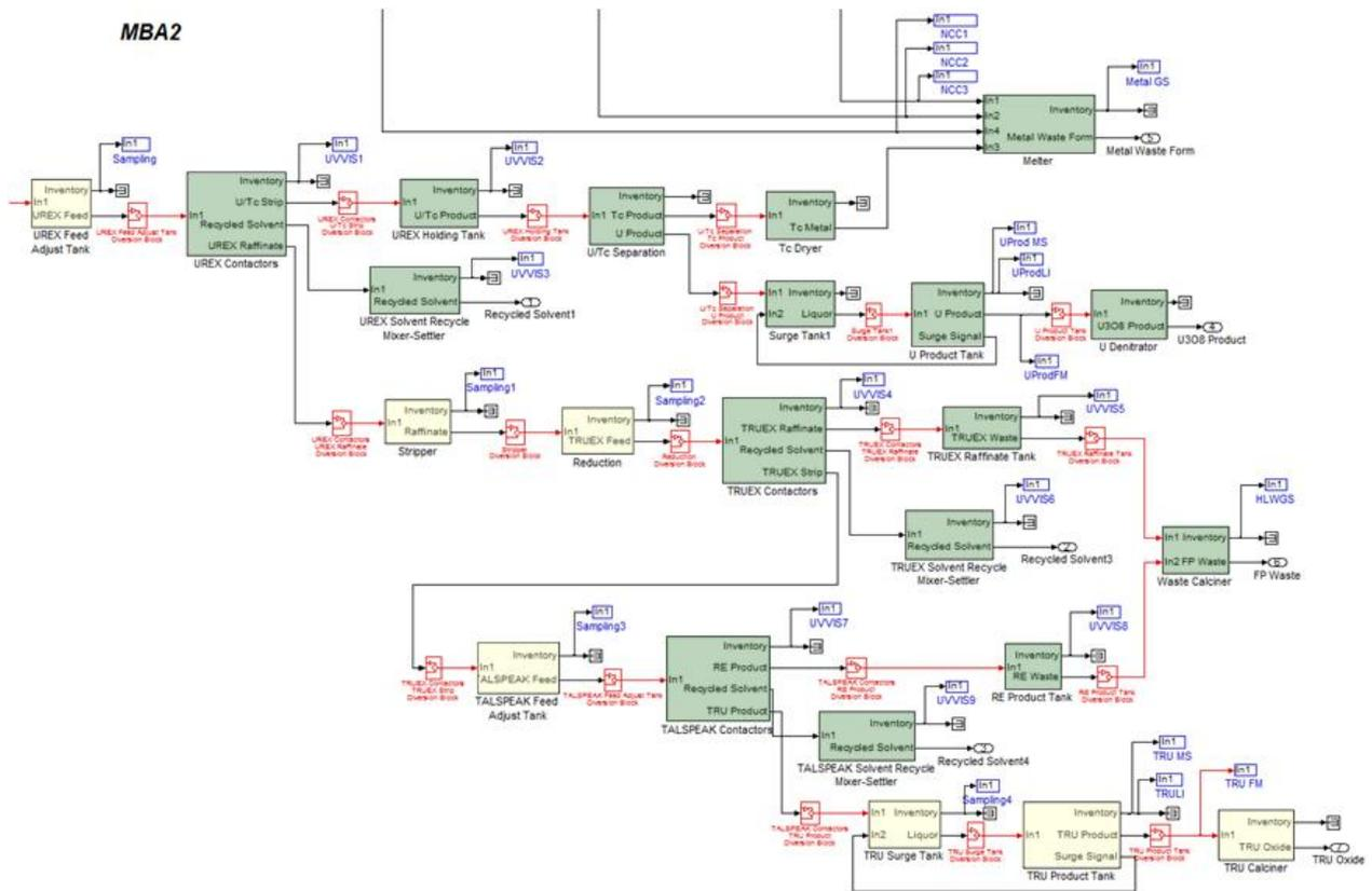
**Figure 11: MBA2 with areas processing small (green) and large (yellow) quantities of plutonium**
