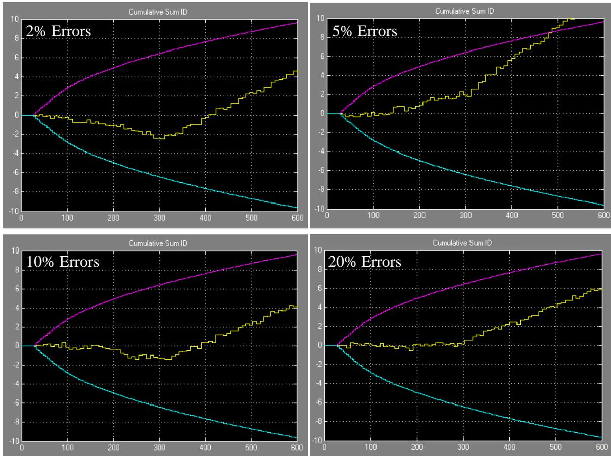
**Figure 12: Parametric analysis results showing little difference in error bars as the uncertainty increases for areas processing small quantities of plutonium**
