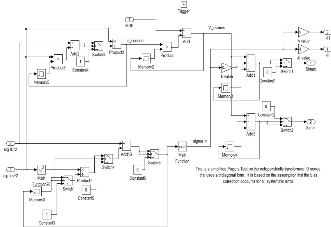
**Figure 4: Simplified Page's Test subsystem**
