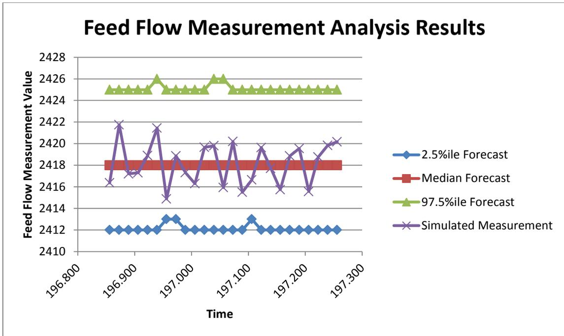
**Figure 8: Bayesian approach, simulated feed flow measurement data and forecasting**
