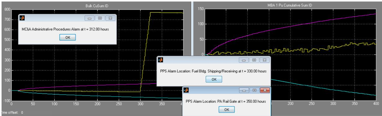
**Figure 23: Abrupt diversion from MBA1 with integrated systems—the administrative procedures alarm triggers an alert state causing two PPS alarms**
