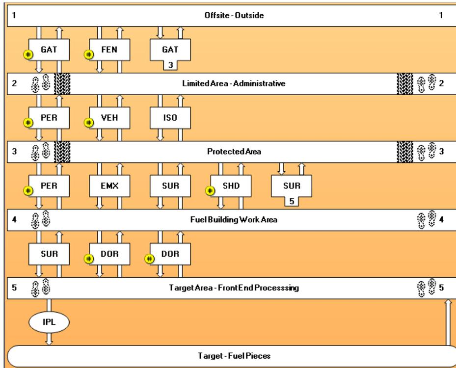
**Figure 13: Adversary sequence diagram for the front end**
