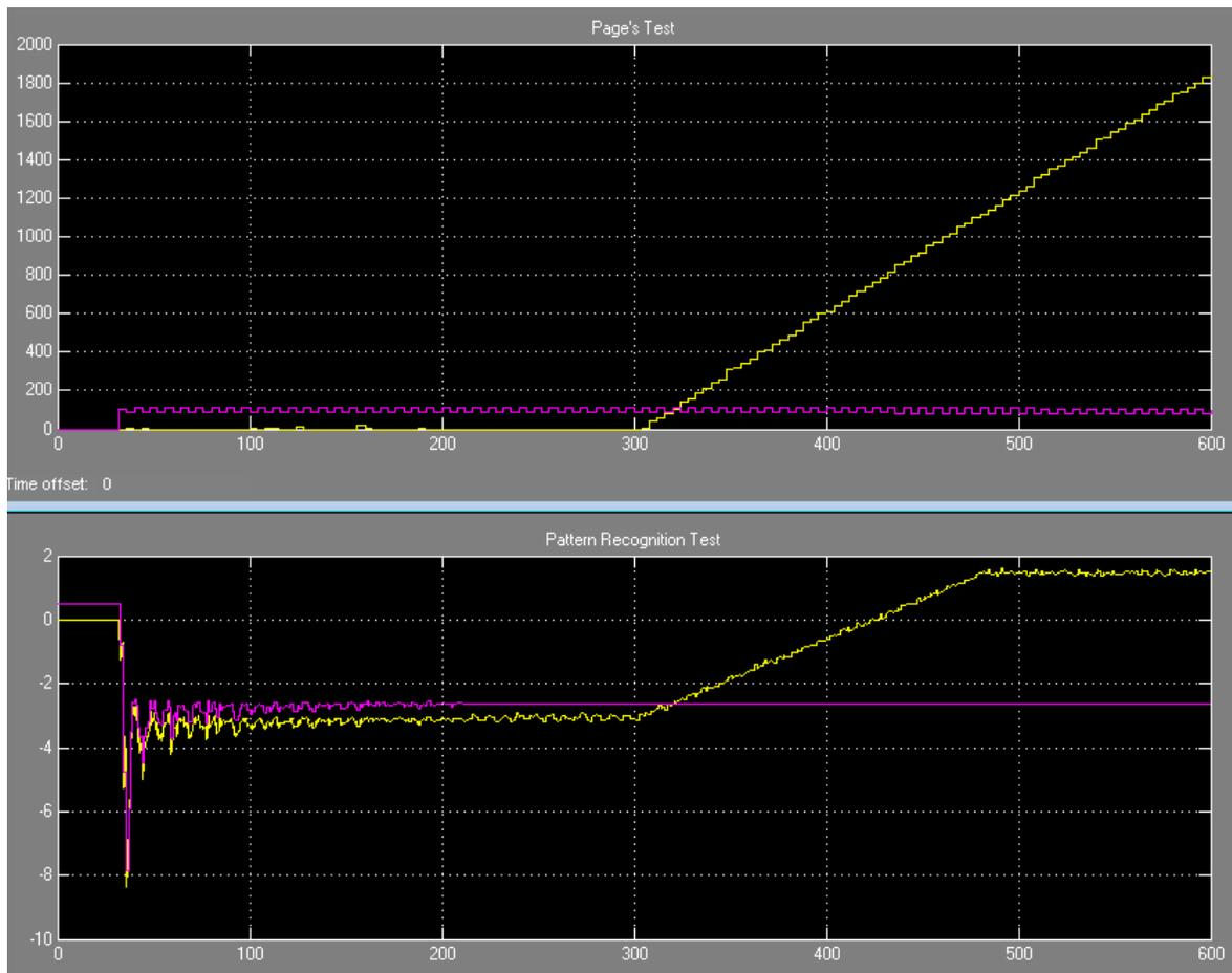
Figure 5: Abrupt diversion response, Page's Test (top), pattern recognition (bottom)
