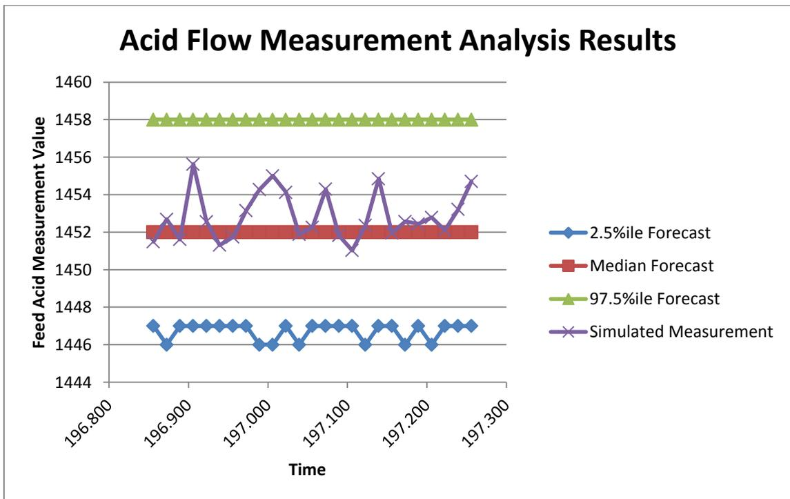
**Figure 9: Bayesian approach, simulated acid flow measurement data and forecasting**
