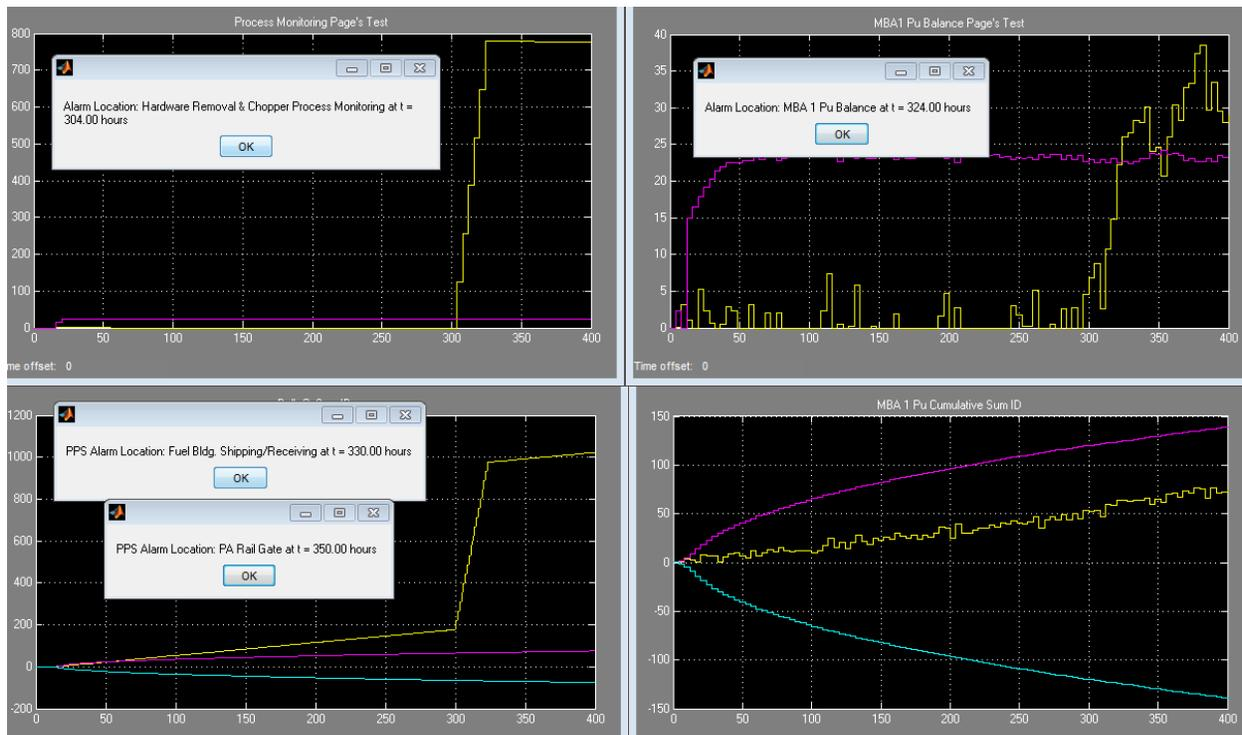
**Figure 20: Abrupt diversion from MBA1 with integrated systems—the process monitoring alarm triggers an alert state causing two PPS alarms**
