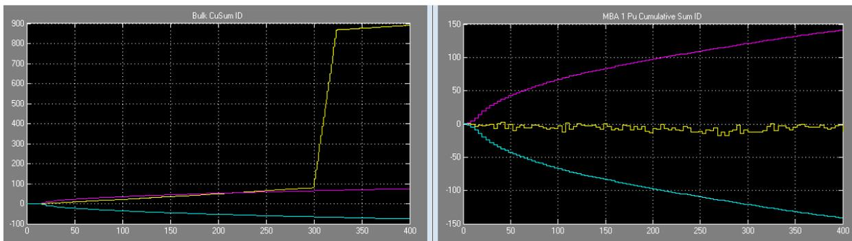
**Figure 19: Abrupt diversion from MBA1 without integrated systems—no PPS alarm blocks were indicated during the diversion**
