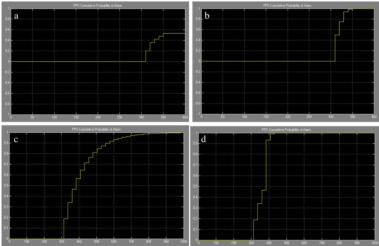
**Figure 25: Cumulative probability of detection in the PPS elements for (a) abrupt diversion without integrated systems, (b) abrupt diversion with integration, (c) protracted diversion without integration, (d) protracted diversion with integration.**
