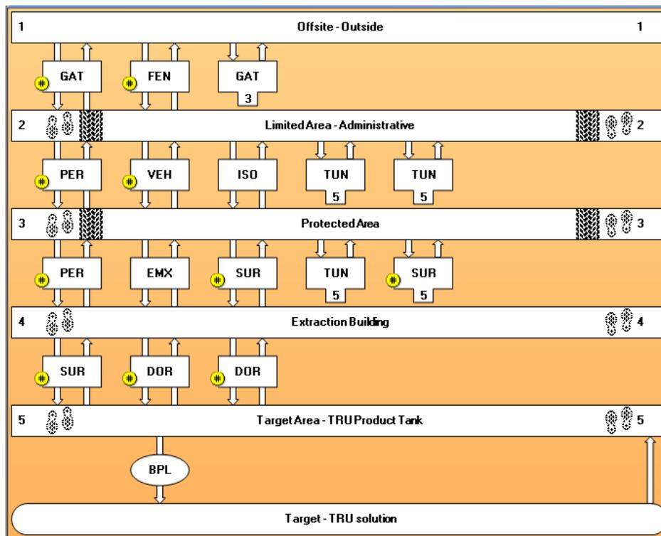
Figure 14: Adversary sequence diagram for separations
