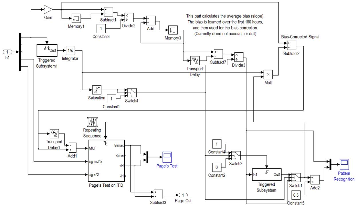
Figure 3: Bias correction and alarm subsystem
