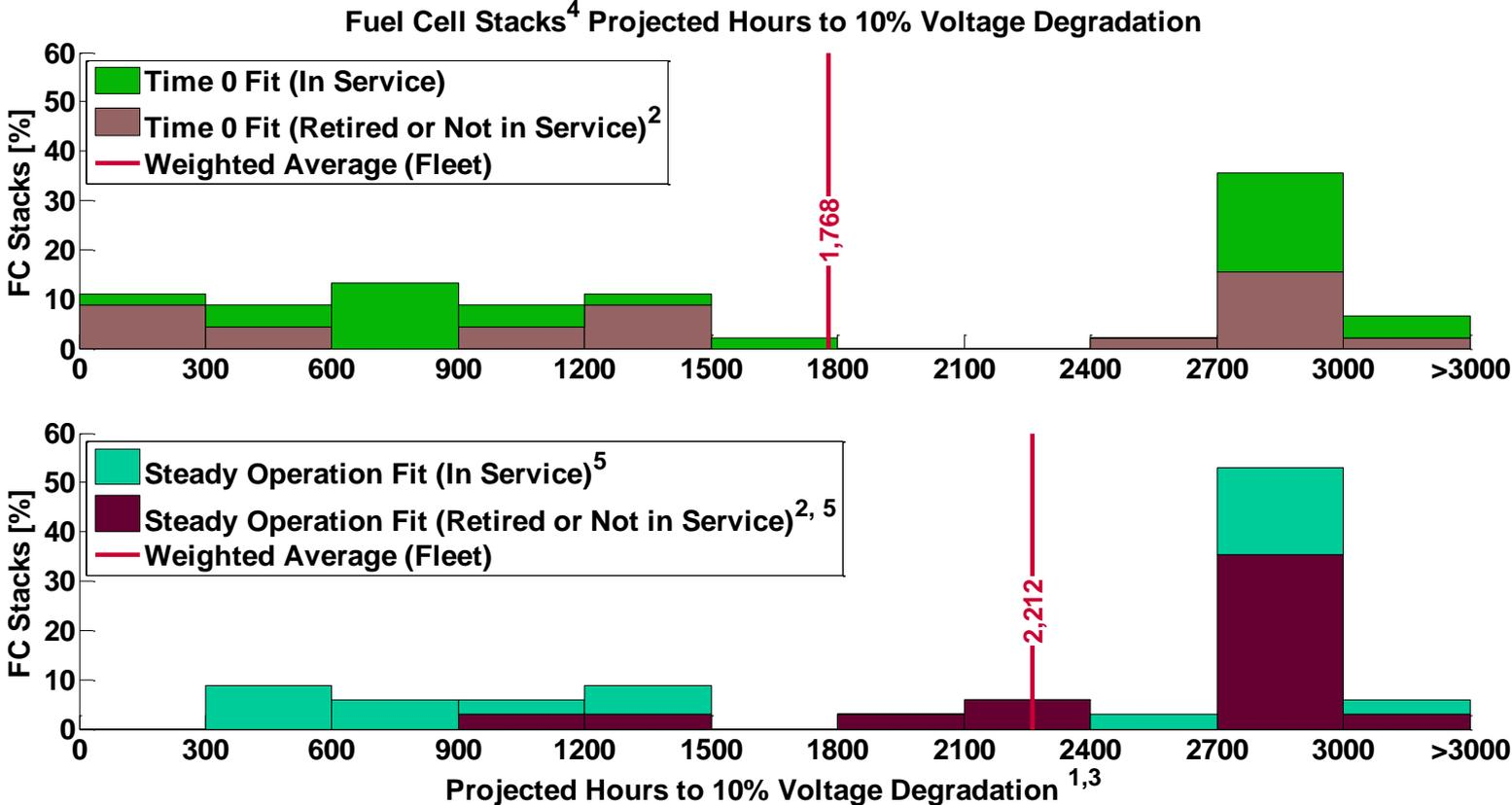
1) Projection using field data, calculated at high stack current, from operation hour 0 or a steady operation period. Projected hours may differ from an OEM's end-of-life criterion and does not address "catastrophic" failure modes.
