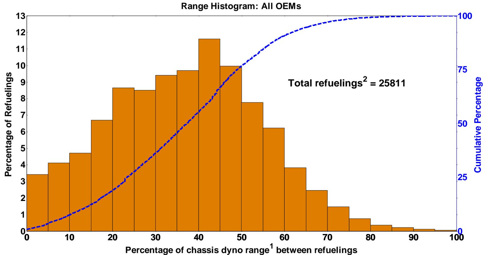
1. Range calculated using the combined City/Hwy fuel economy from dyno testing (not EPA adjusted) and usable fuel on board.
