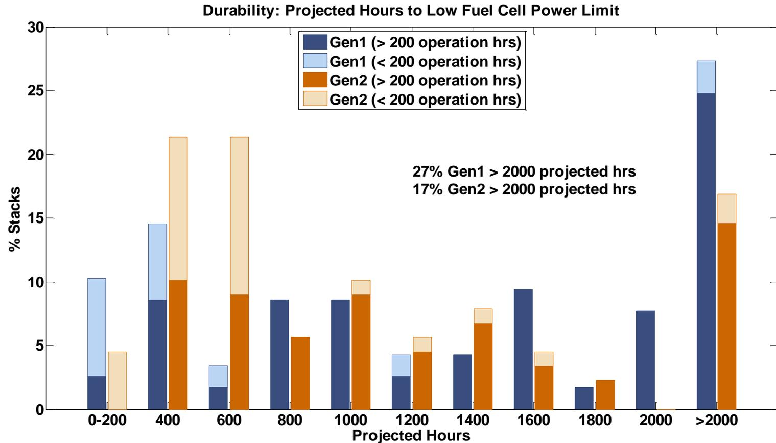
1. Low fuel cell power limit is dependent on the fuel cell vehicle system and is unique to each company in this Learning Demonstration.
