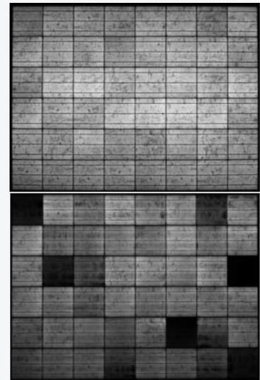
*Electroluminescence imaging of a multicrystalline module before stress testing (top) and after (bottom) at 50°C, 85% relative humidity, and -600 volts for 89 hours. Some cells in the stressed module are dark because of degraded diode characteristics. Image by Stephen Glick, NREL*
