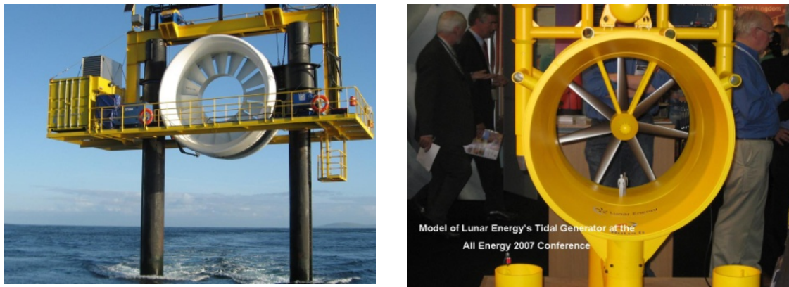
Figure 2: Examples of ducted or shrouded parallel axis lifting surface type turbines (Left to right: OpenHydro turbine being test at EMEC, Lunar Energy turbine)
