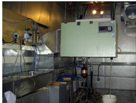
Figure 1. Instrumented outdoor unit (left) and instrumented indoor unit (right) covered by insulated discharge plenum
