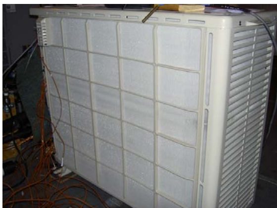
Figure 11. Fujitsu 12LRS outdoor coil immediately prior to defrost operation (left) and outdoor coil immediately following defrost operation (right)
