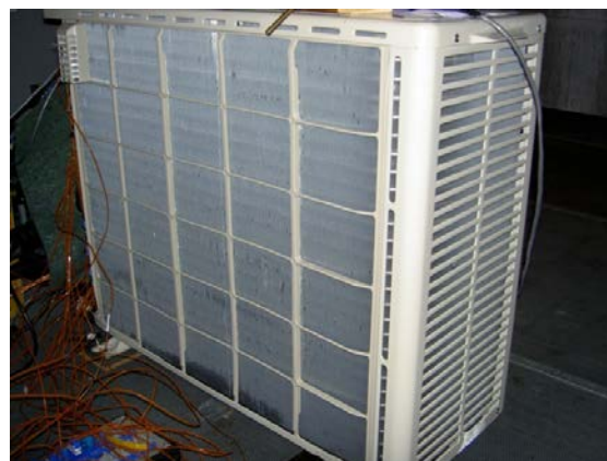
Figure 11. Fujitsu 12LRS outdoor coil immediately prior to defrost operation (left) and outdoor coil immediately following defrost operation (right)
