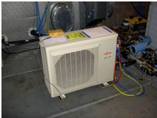
Figure 1. Instrumented outdoor unit (left) and instrumented indoor unit (right) covered by insulated discharge plenum
