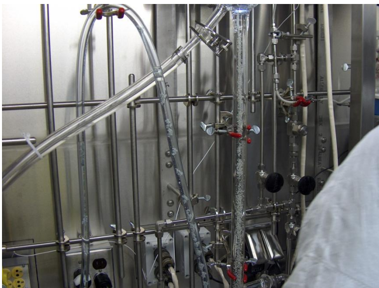
Figure 1. Zr-Y gel spheres with SiC particles in gelation column and associated tubing.
