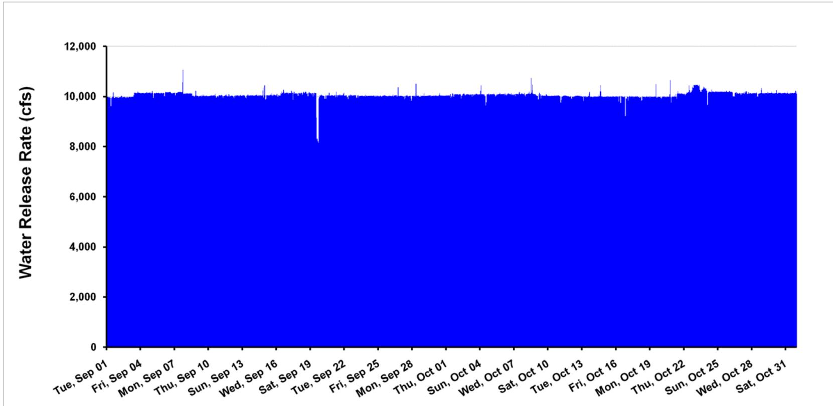
Figure 3.2 Release Pattern of the Fall Steady Flow Conducted in September/October 2009
