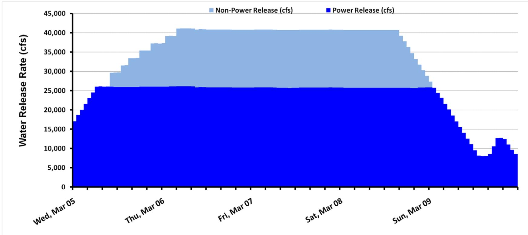
Figure 3.3 Release Pattern of the High Flow Experiment Conducted in March 2008
