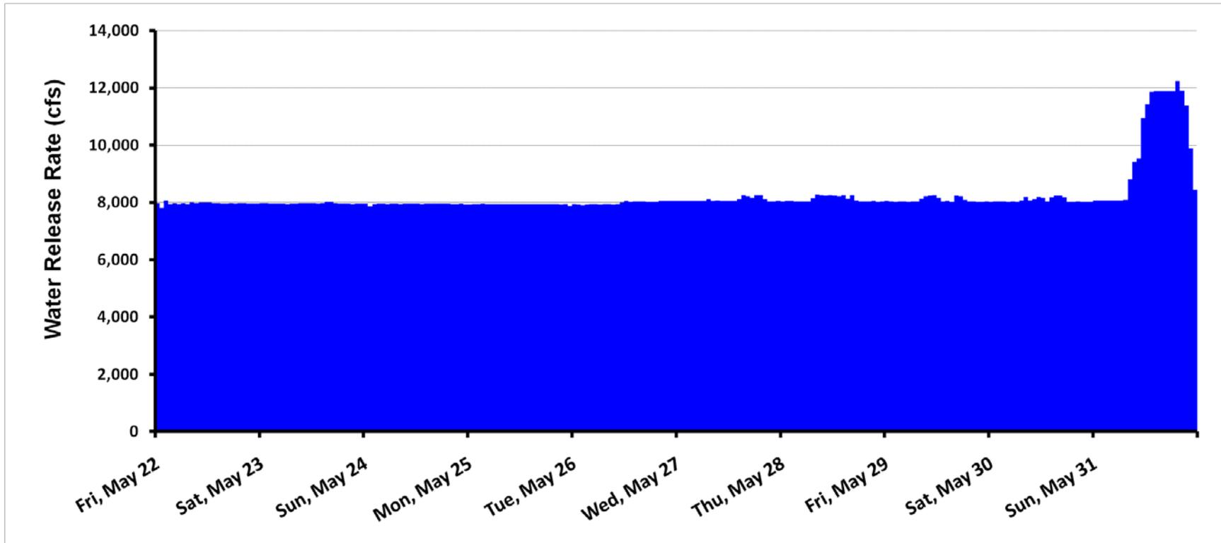
Figure 3.1 Release Pattern for the Aerial Photography Steady Flow Conducted in May 2009
