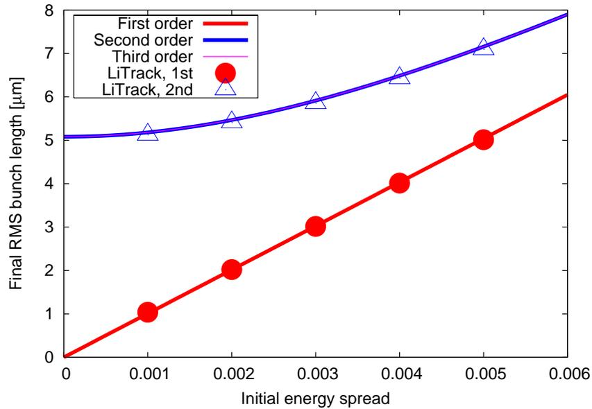
Figure 2: Minimum final bunch length as a function of the initial energy spread, consider up to first, second or third order effects. For a perfectly linearized bunch plus a four bend chicane, the third order effect can be negligible. The optimal compression condition  $1 + h_1 R_{56} = 0$  is fulfilled. Good agreement between the analytical formulae and LiTrack simulation.
