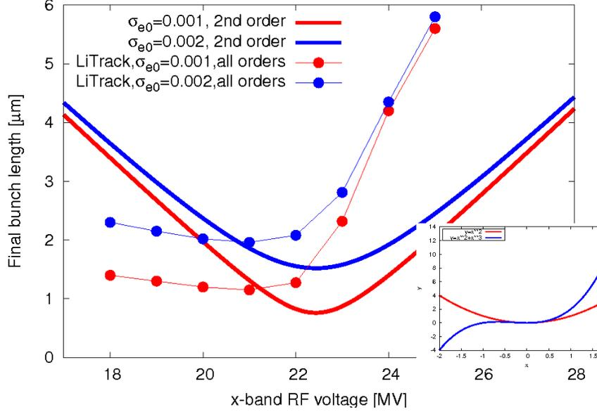
Figure 4: Minimum final bunch length as a function of the x-band RF voltage, for two different initial un-correlated energy spread. Dots represent simulation results from LiTrack where the energy chirp to any order is included, while curves are plotted from formulae (14) and (23) where the terms up to second order is kept.
