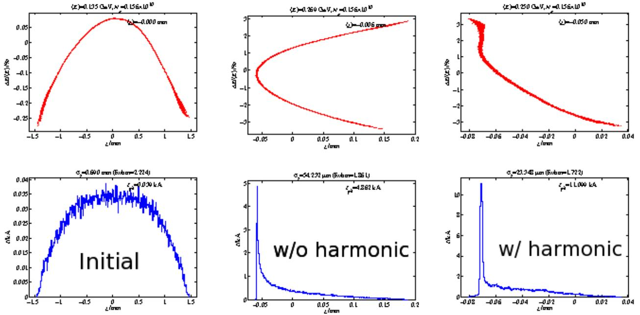
Figure 6: Left: initial beam at a beam energy of 135 MeV; middle: after BC1, without harmonic RF, at a beam energy of 269 MeV, peak current of 5 kA; Right: after BC1, harmonic RF voltage equals 19 MV with a RF phase of -180 degree, at a beam energy of 250 MeV, peak current of 10 kA.
