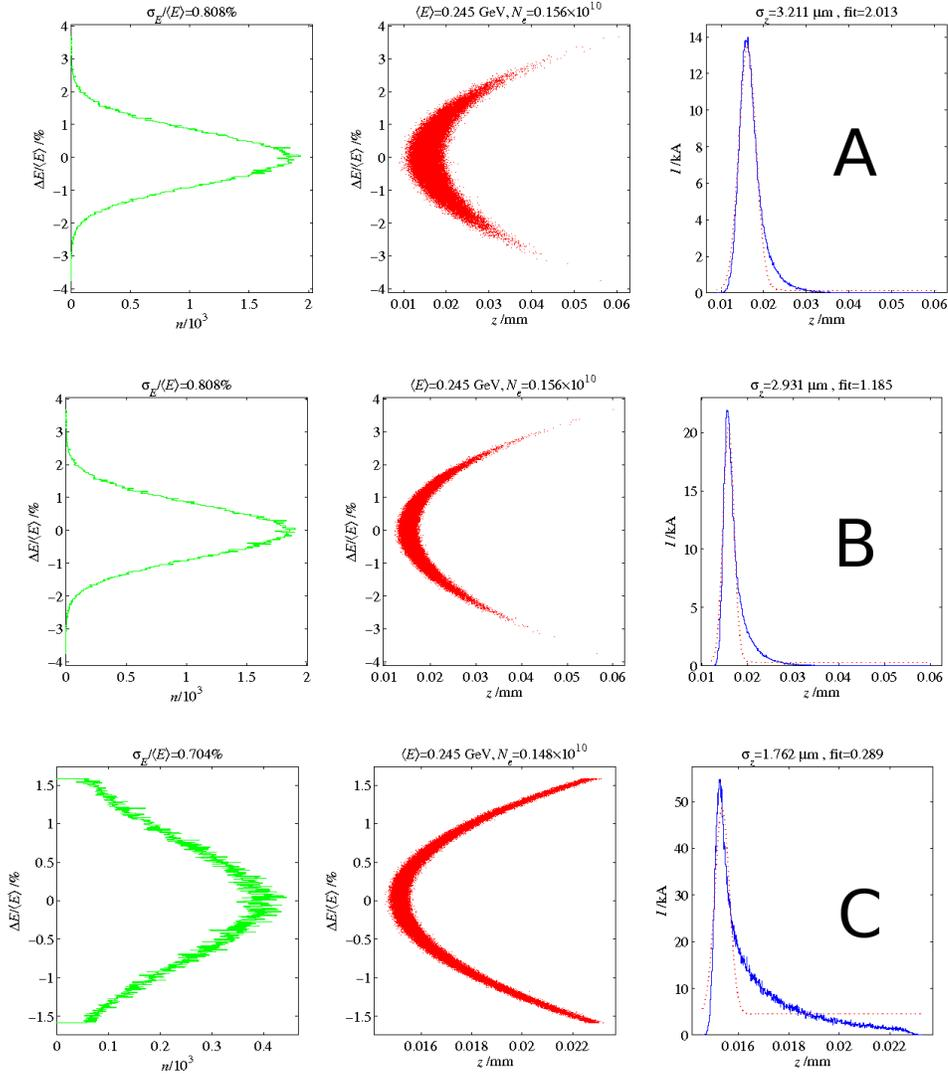
Figure 5: Final longitudinal phase space after chicane for three cases: (A) initial un-correlated energy spread of 0.2%; (B) initial un-correlated energy spread of 0.1%; (C) initial un-correlated energy spread of 0.02%.
