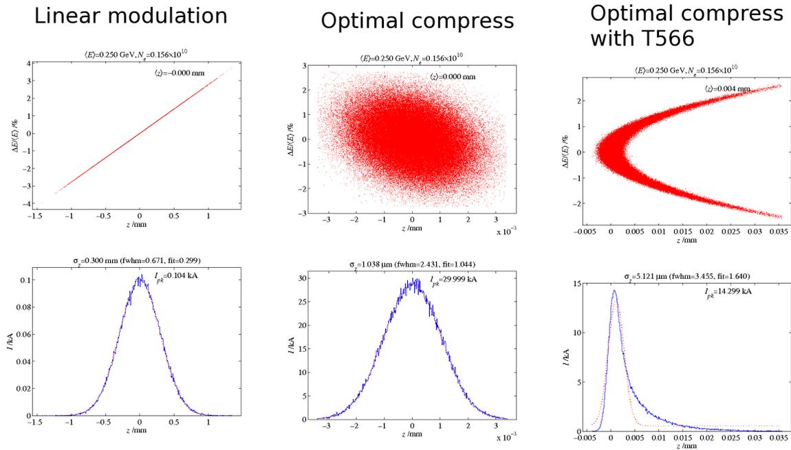
Figure 3: Longitudinal phase space and current (RMS and FWHM fitting bunch length) for 3 cases from Litrack simulation: initial condition with linear energy modulation; optimal compression with only  $R_{56}$ , a final bunch length of  $1\mu m$  (FWHM fit); optimal compression with both  $R_{56}$  and  $T_{566}$ , a final bunch length of  $1.7\mu m$  (FWHM fit).
