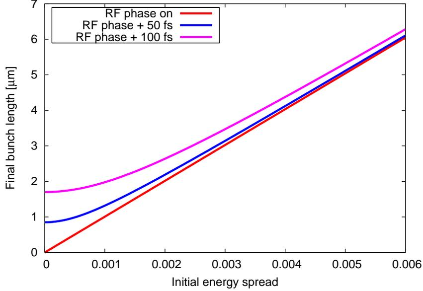
Figure 1: Minimum final bunch length as a function of the initial energy spread, without or with RF phase jitter.
