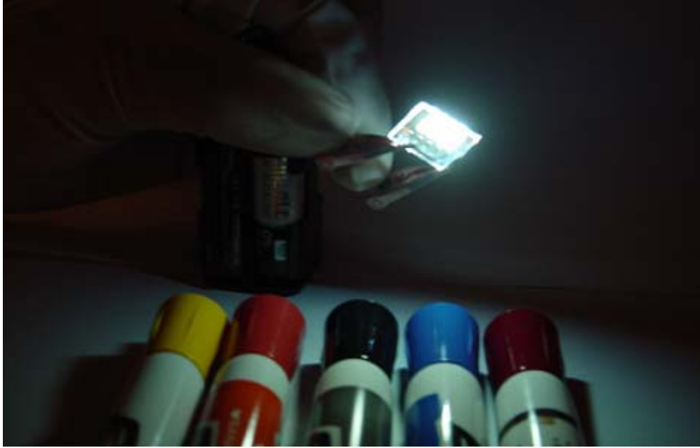
Figure 8: Agiltron's white OLED device with an excellent color rendering index of over 75.
