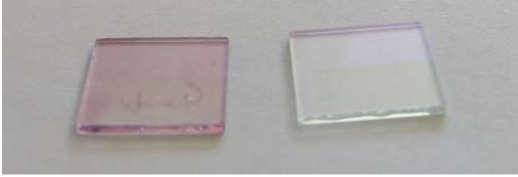
Figure 2: Au (left) and ITO (right) NP coated ITO substrates.
