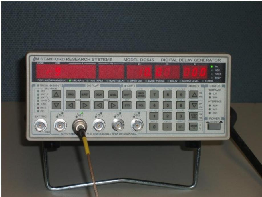
Figure 7: Stanford Research Systems Digital Delay Generator (Model DG645).
