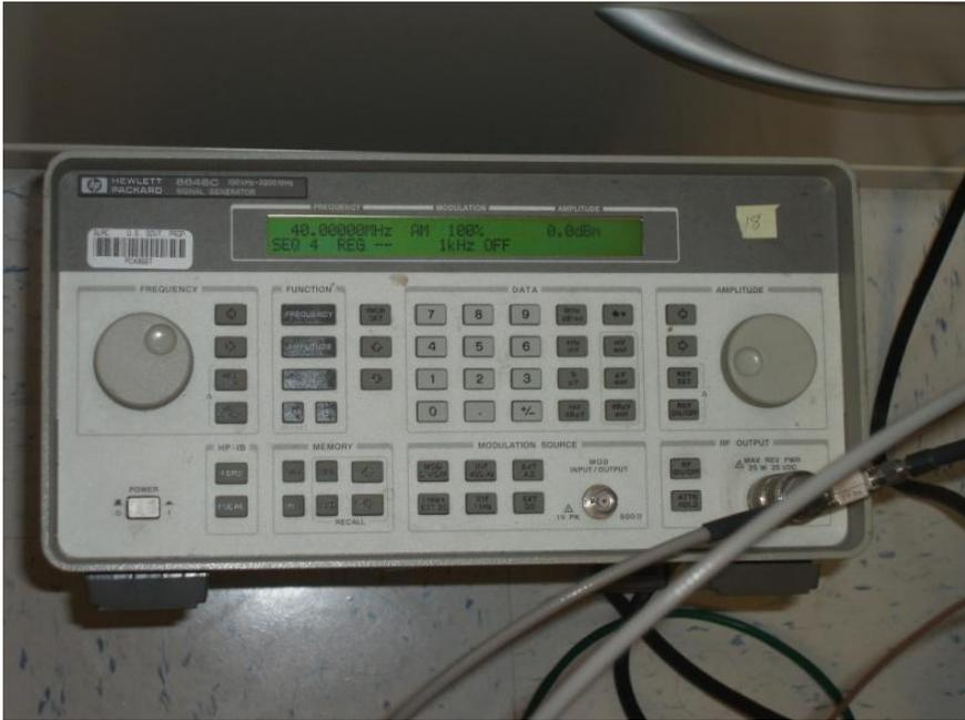
Figure 6: An HP Signal Generator (Model 8648C)
