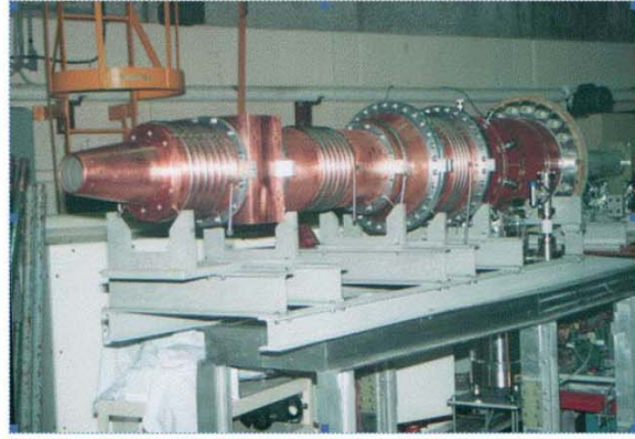
Figure 1: (Right) An assembled view of the CT injector. All plasma facing components are coated with state-of-the-art high quality coating of dense tungsten to reduce electrode erosion. It has shown clean metallic-impurity-free fuelling of TdeV. Shown on the left is the capacitor bank power supply used for forming the CT. A similar (but larger) capacitor bank (not shown here) is used to accelerate the CT. All these, including the vacuum systems and CT diagnostics are presently in storage at PPPL.
