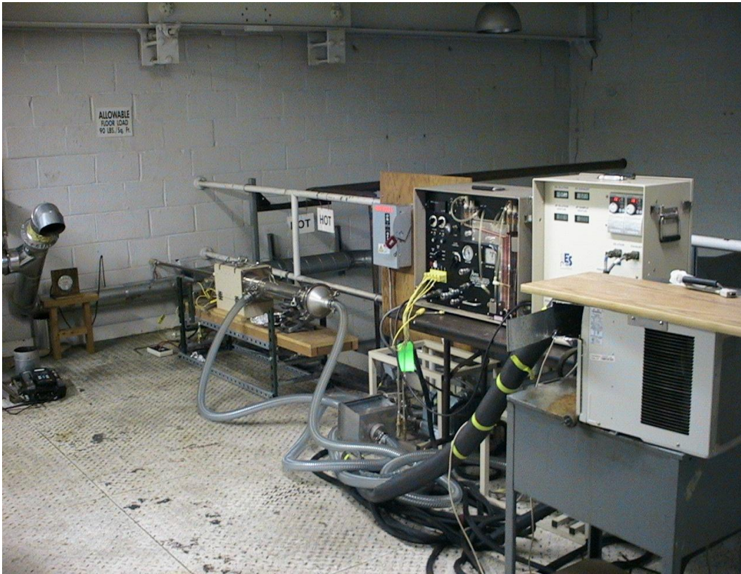
Figure 12. Particulate Sampling and measurement System
