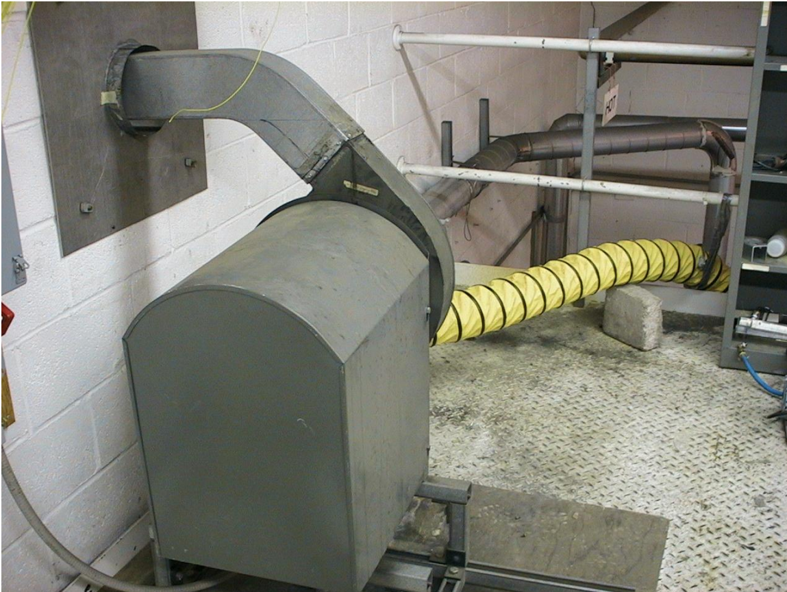
Figure 11. Sampling Stack with Induced Draft Fan
