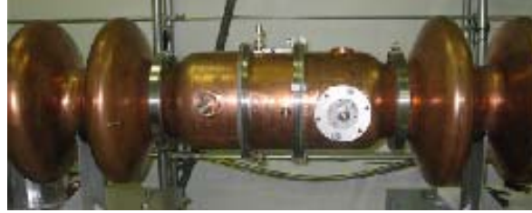
FIG. 16: Connecting tube with damper ring
