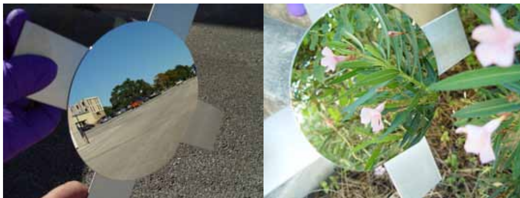
Figure 42. Photographs of deposited films exhibiting high specular reflectance.
