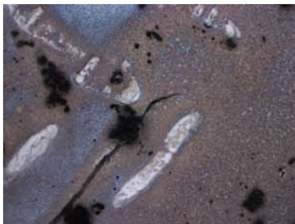
Figure 126. Crack tip on supported side of the membrane, 500X, BF, Membrane #2. Software was used to capture and compile several images through multiple focal planes, resulting in some pixilated regions. The dark spots are voids.
