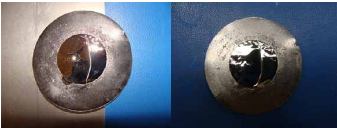
Figure 142. Crack in Pd-128 following testing.
