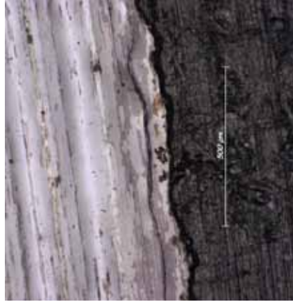
Figure 124. Another crack along the gasket.
