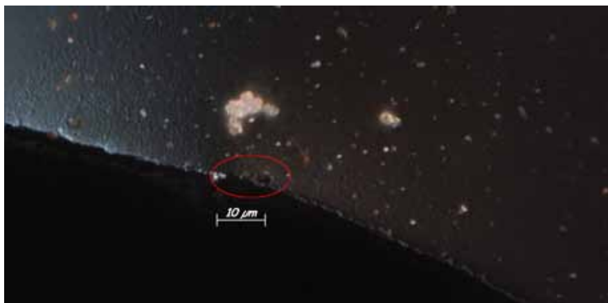
Figure 119. View of a possible defect along the crack edge, at 1000X, C-DIC, Membrane #1.
