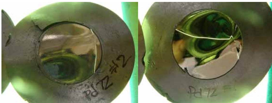
Figure 117. Feed-side of membranes #1 and #2, shown with back-lighting to easily identify cracks.
