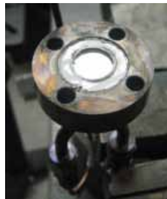
Figure 114. Membrane loaded into fixture.
