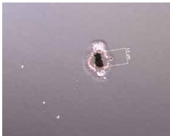
Figure 129. An atypical pit with precipitate around the periphery, 500X, C-DIC, new foil sample.
