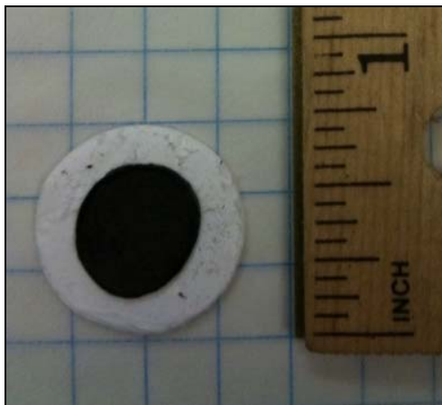
Figure 1. Digital photograph of a cathode composed of electrospun, Chevrel phase \text{Mg}_2\text{Mo}_6\text{S}_8 loaded carbon fibers. The green fibers were punched into \frac{3}{4} " disks that shrank down to approximately \frac{1}{2} " during heat treatment.
