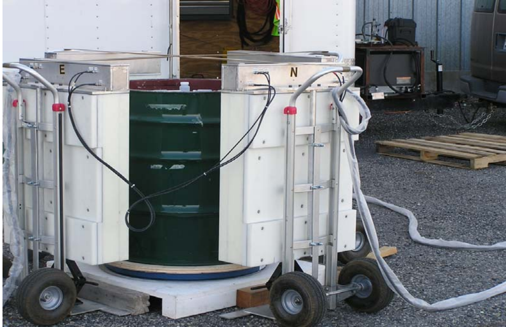
Figure 3.2. Measurements of the test drum with ^{252}\text{Cf} source inside
