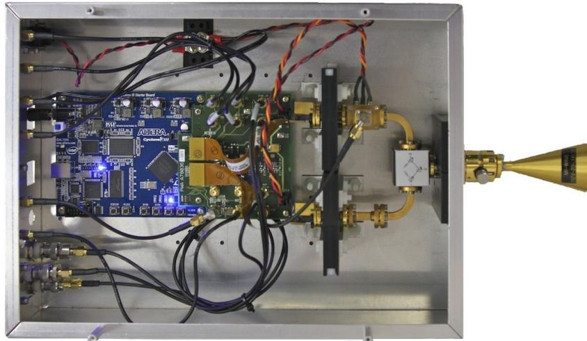
**Figure 16.** One of the millimeter-wave transceivers used in the full-duplex, key-generation system. The transceiver consists of an FPGA, interface board, parallel transmitter and receiver, and a waveguide front end with horn antenna.
