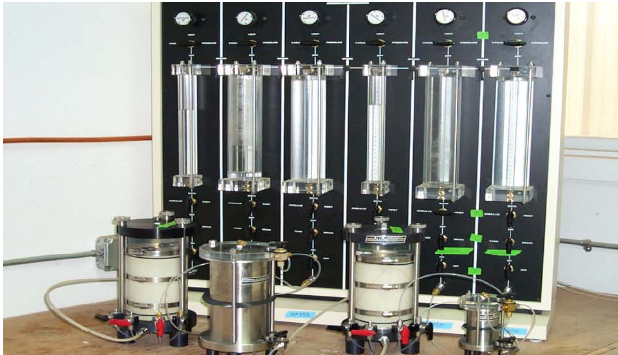
Figure 5 Flexible-walled Permeameter Apparatus.
