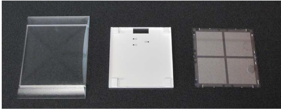
Figure 11: The three components that make up the OLED lamp; from left to right, lens, lamp mounting frame and the OLED light plate.
